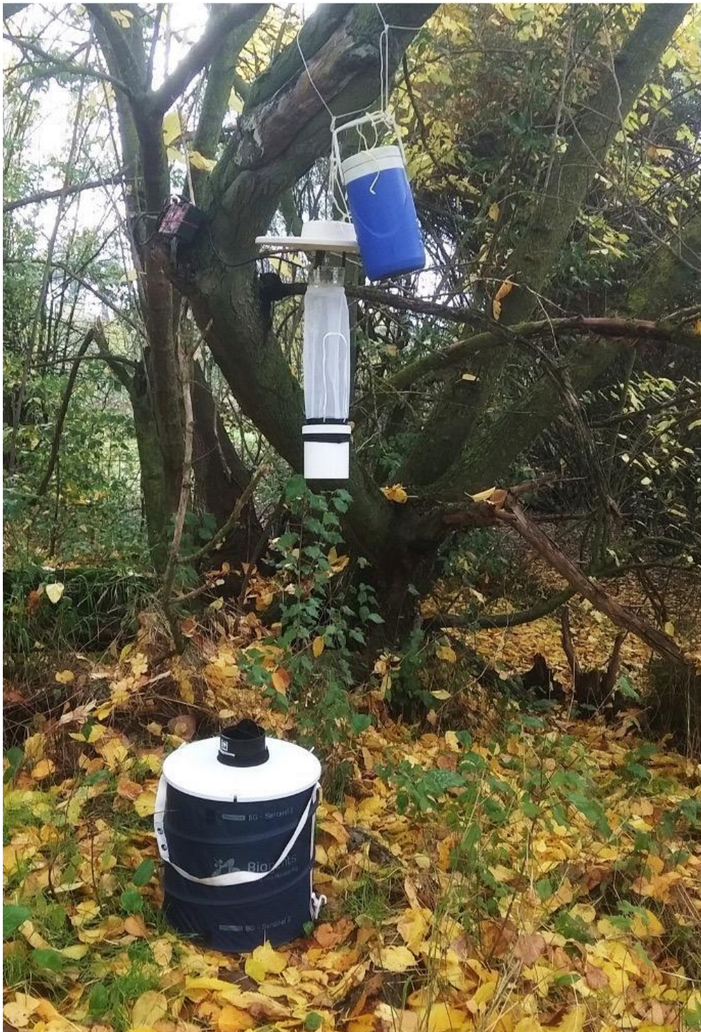
Supplementary Figure 1. Mosquito trapping station including a CDC-type miniature white light trap at 1.8 m from the soil, a BG sentinel trap on soil and the CO 2 deliver device on top of the traps (2.2m height).
